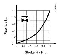
$\begin{array}{ccc} 0...30~\% & \rightarrow & linear \\ 30...100~\% & \rightarrow & equal~percentage \\ & & n_{gl} = 3~as~per~VDI~/~VDE~2173 \end{array}$
