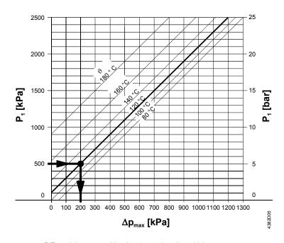
$\Delta p_{\text{max}}$  = Differential pressure with valve almost closed, at which cavitation can largely be avoided
