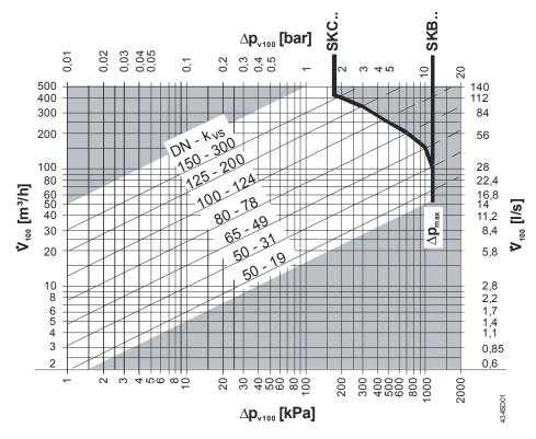
$\Delta p_{max}$  = Maximum permissible differential pressure across the valve, valid for the entire actuating range of the motorised valve
